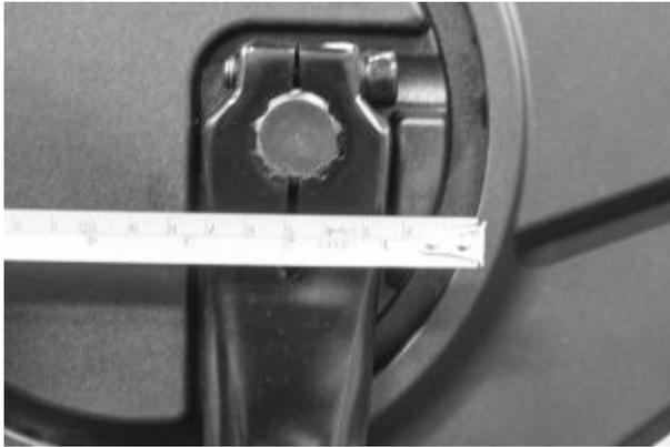
rogue went with a wildly overbuilt crank arm that attaches via compression fitting over a fluted rod.
