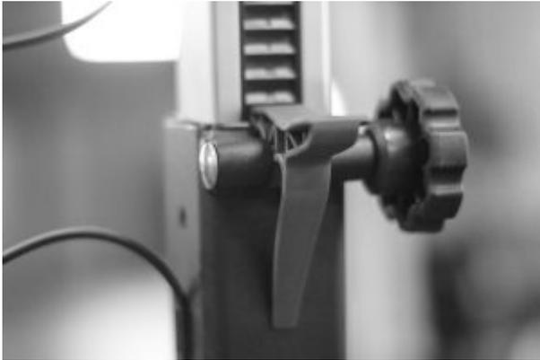
c2 has this fast cam styled adjuster for the seat post and handle bar - if the crank is loosened you can pull the bars or seat up easily and it will not slide down, then just tighten it at what ever level you like.
