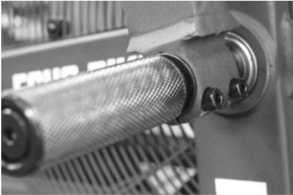
rogue also put the pedal/swing arm linkage bars inside the fan cage, and attached the handles via the same fluted rod/grooved compression system that gives an incredibly solid feel that shouldn't shake loose through regular use.
