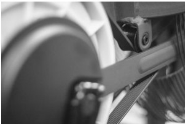
close up of one of the belt tensioners
