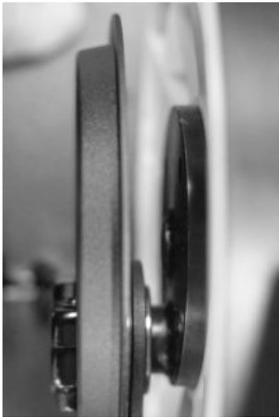
this is an above shot of the rogue bike after the shroud has been removed - you can see the crank arm on the left at the bottom - on the other side of the plastic guard is a circular steel plate - looks about 4" in diameter and at least 1/4" thick that the fluted rod is welded to, effectively eliminating all the crank arm problems with the other 2 airbikes.
